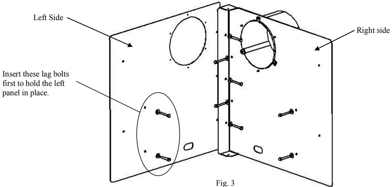
**STEP 3:** Attach the wall plate to the wall with the pass through heat-shields in place and fasten to the wall using the 9 lag bolts provided. Mount the left side first with the 2 outer lag bolts, then mount the right side. See Fig. 3.
