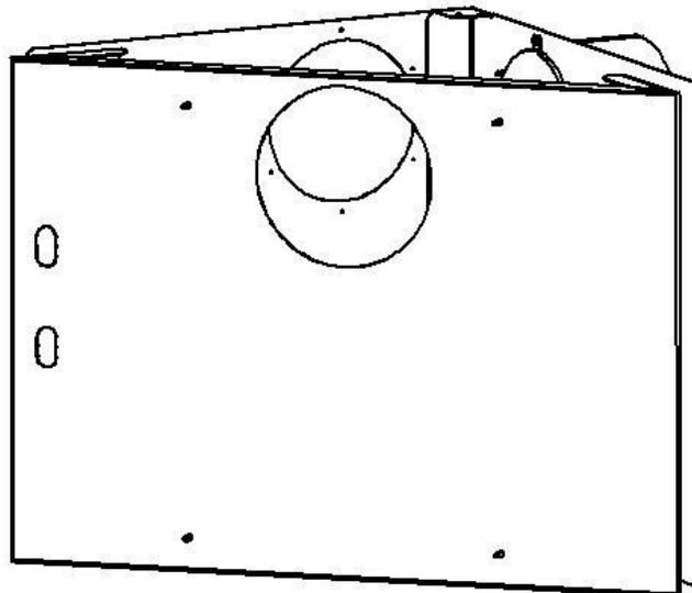
**Step 4:** Having secured the wall plate to the wall, fit the diagonal mounting plate as shown in Fig. 4. Please ensure that all four mounting pins are fully engaged in the 4 keyway slots.
